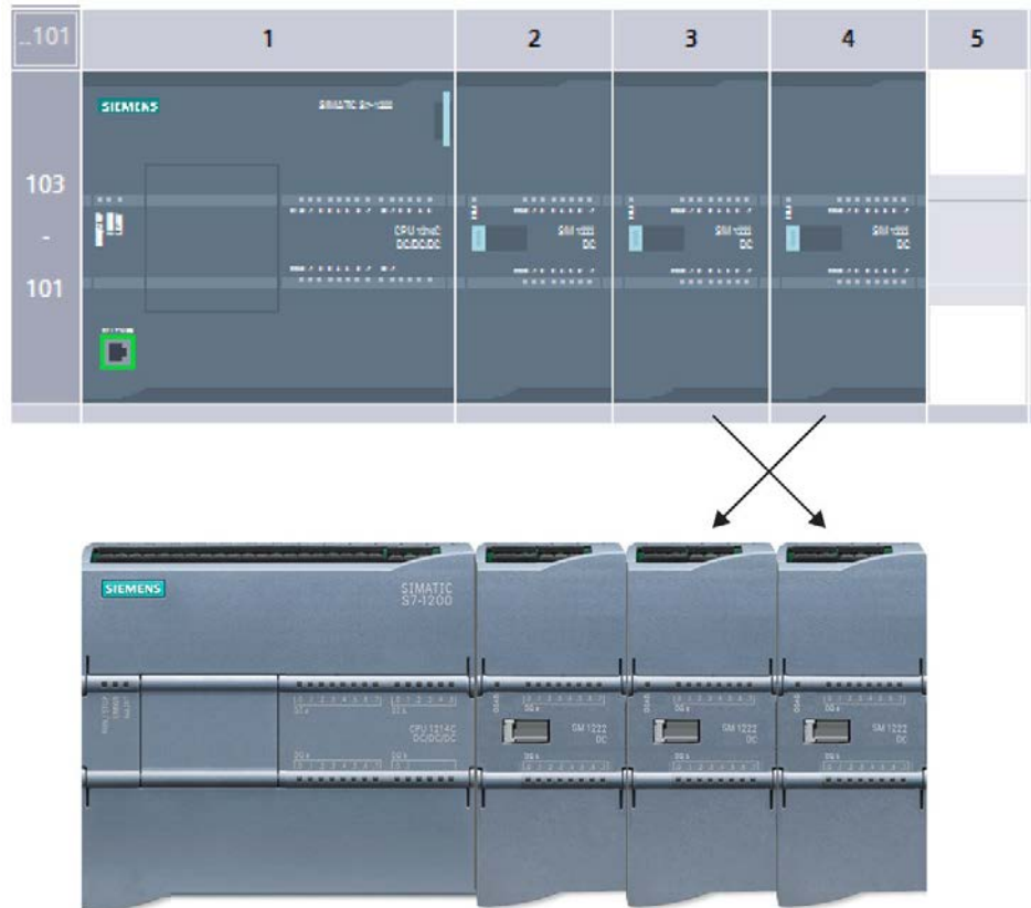
Figure 6-3 Device configuration compared to actual installation with modules in slots 3 and 4 swapped
